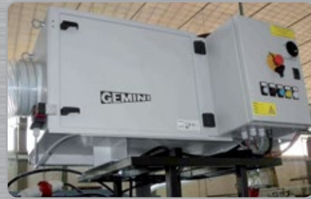
Electrostatic filtration system
